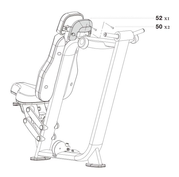
**STEP 20** SECURELY tighten all bolt connections.
