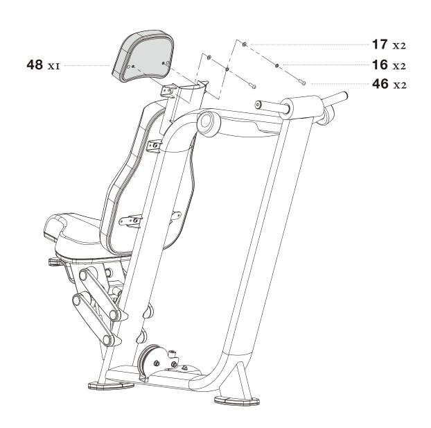
**STEP 17** SECURELY tighten all bolt connections.
