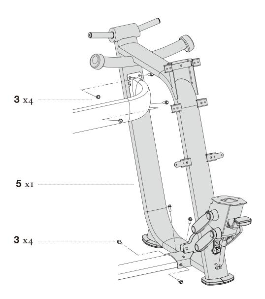
**STEP 4** SECURELY tighten all bolt connections.
