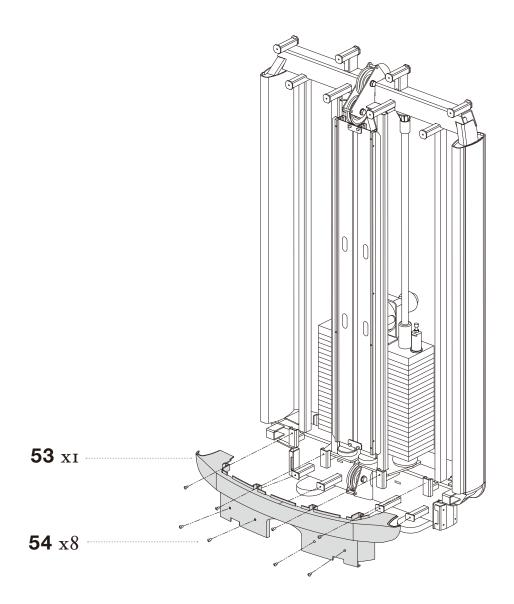
**STEP 22** SECURELY tighten all bolt connections.
