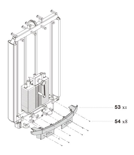
**STEP 21** SECURELY tighten all bolt connections.
