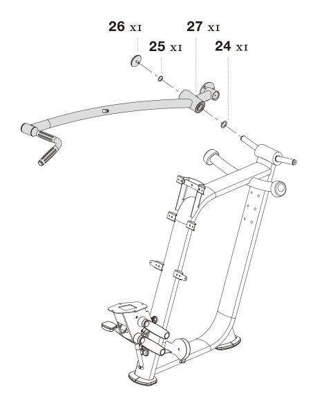
**STEP 8**SECURELY tighten all bolt connections.
