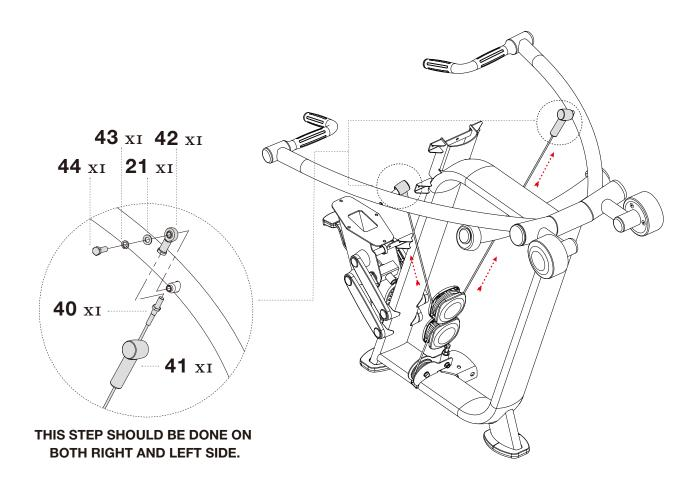
**STEP 14** SECURELY tighten all bolt connections.
