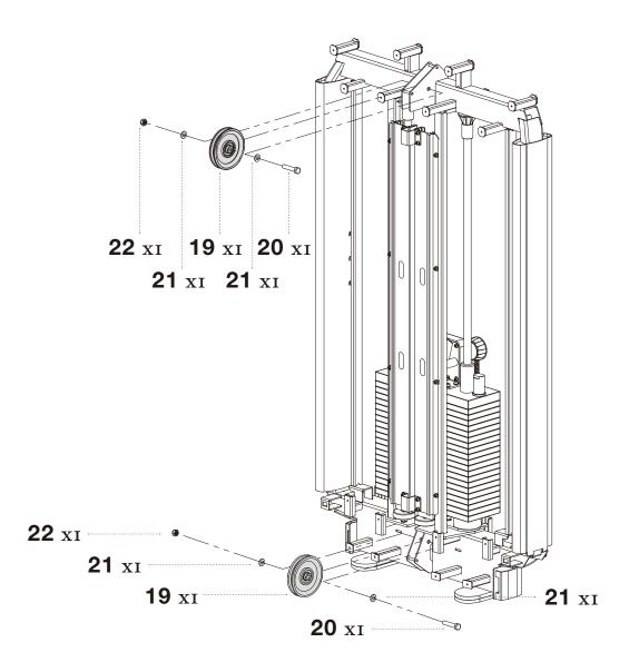
**STEP 6** SECURELY tighten all bolt connections.
