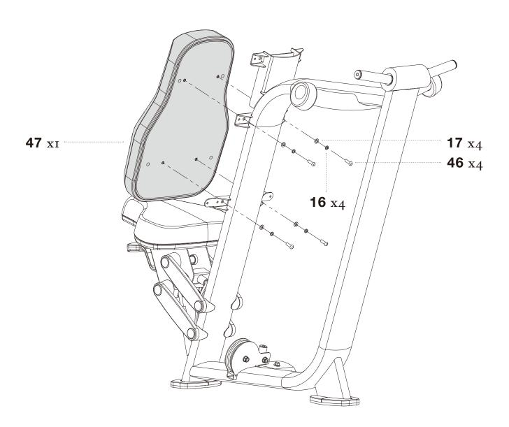
**STEP 16** SECURELY tighten all bolt connections.
