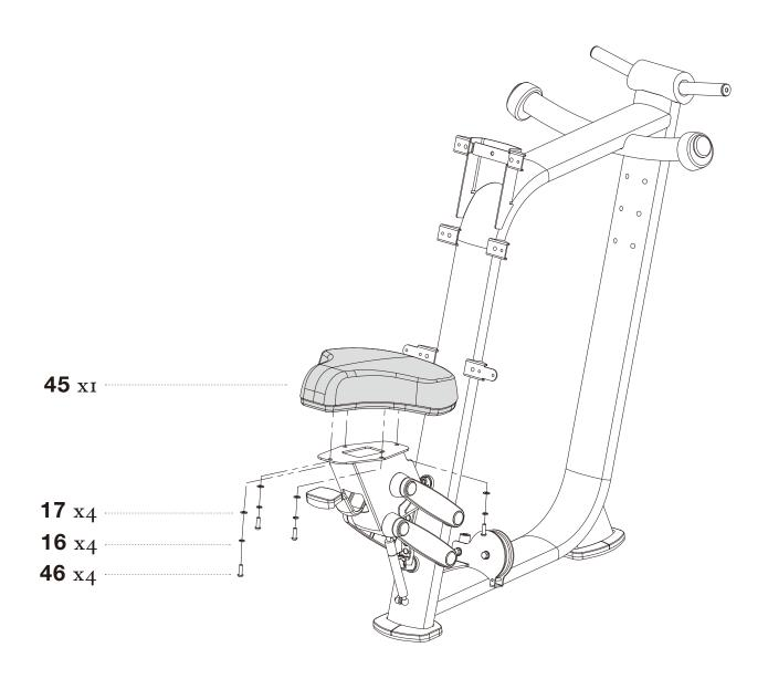
**STEP 15** SECURELY tighten all bolt connections.
