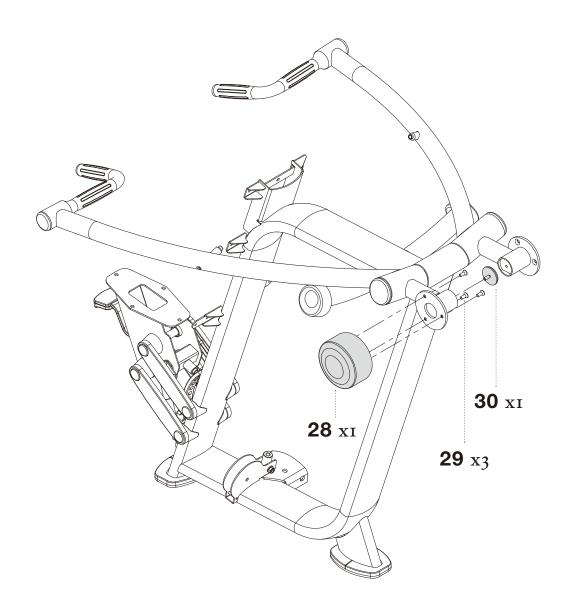
**STEP 9** SECURELY tighten all bolt connections.
