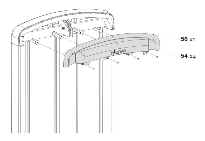
**STEP 25** SECURELY tighten all bolt connections.
