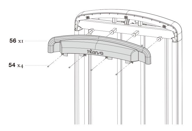
**STEP 24** SECURELY tighten all bolt connections.
