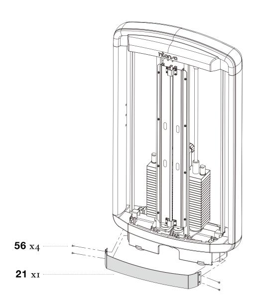
**STEP 31** SECURELY tighten all bolt connections.
