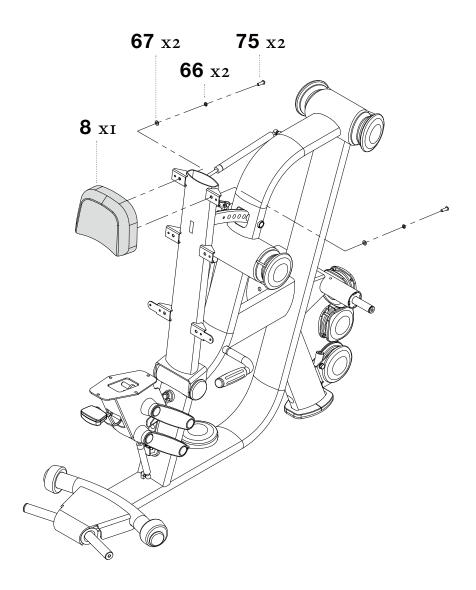
**STEP 22** SECURELY tighten all bolt connections.
