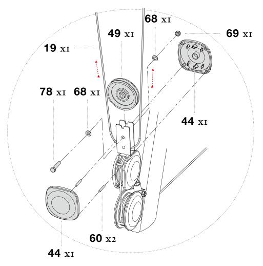
**STEP 18** SECURELY tighten all bolt connections.
