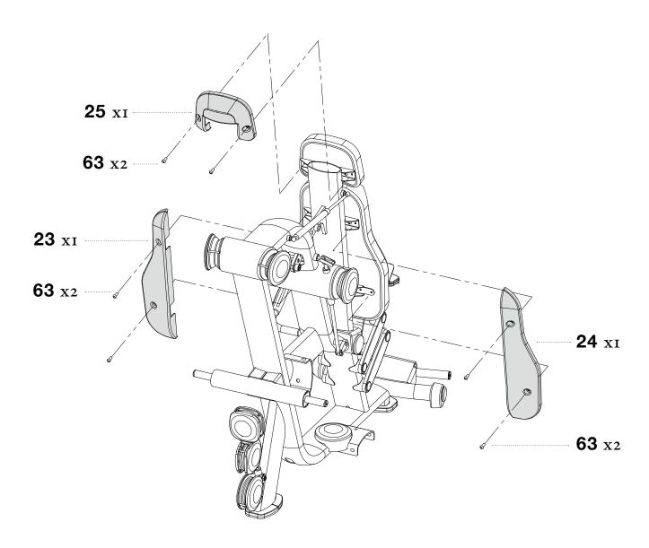
**STEP 24** SECURELY tighten all bolt connections.
