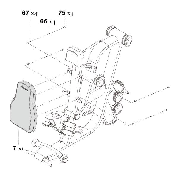
**STEP 23** SECURELY tighten all bolt connections.
