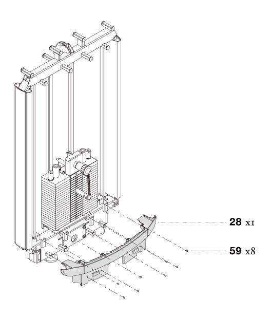
**STEP 26** SECURELY tighten all bolt connections.
