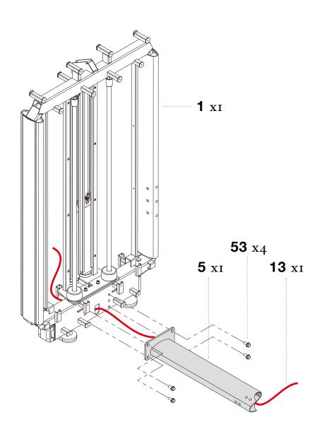
**STEP 2**LOOSELY fasten the bolt connections in this step. Do not fully tighten.
