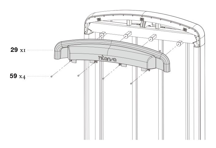
**STEP 29** SECURELY tighten all bolt connections.
