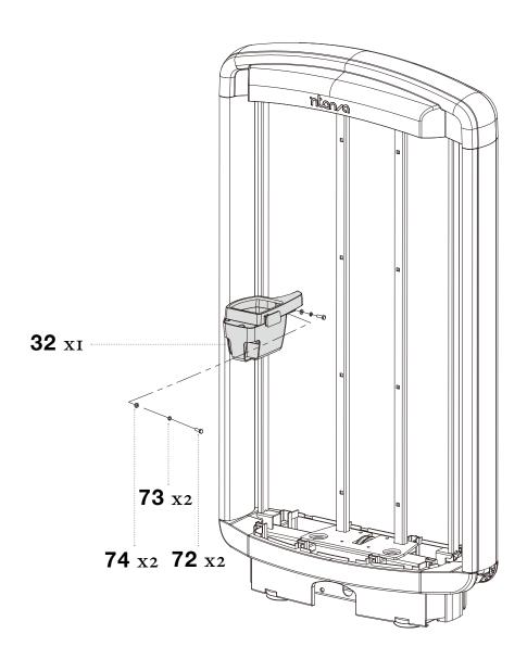
**STEP 35** SECURELY tighten all bolt connections.
