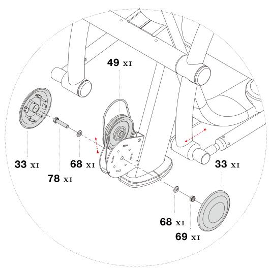
**STEP 15** SECURELY tighten all bolt connections.
