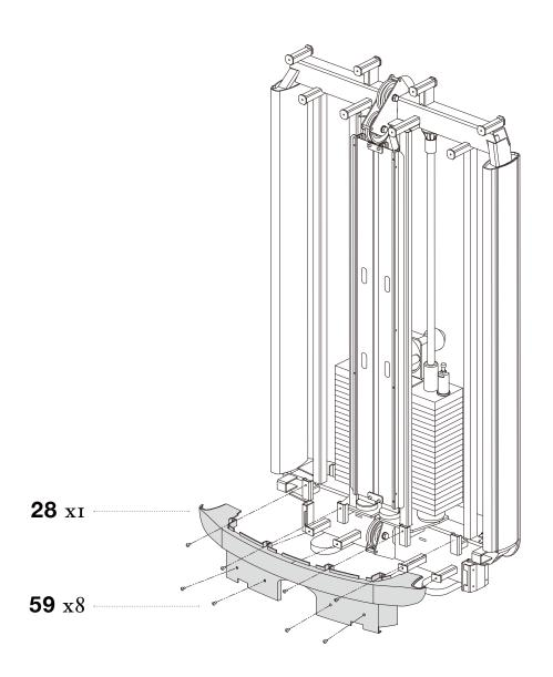
**STEP 27** SECURELY tighten all bolt connections.
