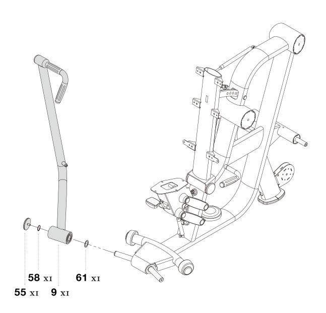
**STEP 9** SECURELY tighten all bolt connections.
