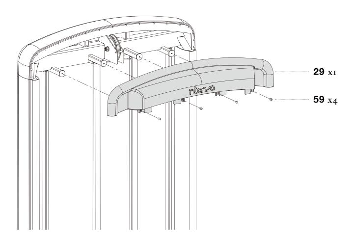
**STEP 30** SECURELY tighten all bolt connections.
