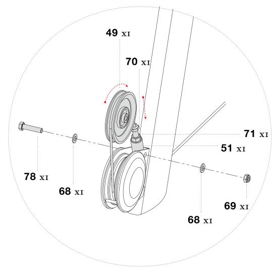
**STEP 16** SECURELY tighten all bolt connections.
