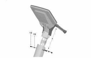
INSTALLING THE 550ETe2 CONSOLE—ASSEMBLE THE CONSOLE. COMPONENTS AND TOOLS
